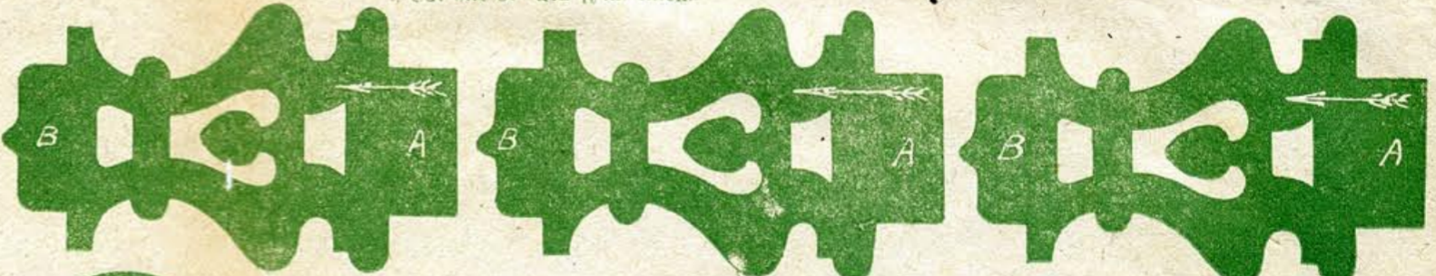
UPRIGHTS. Cut one of each 1/4 in. thick.
