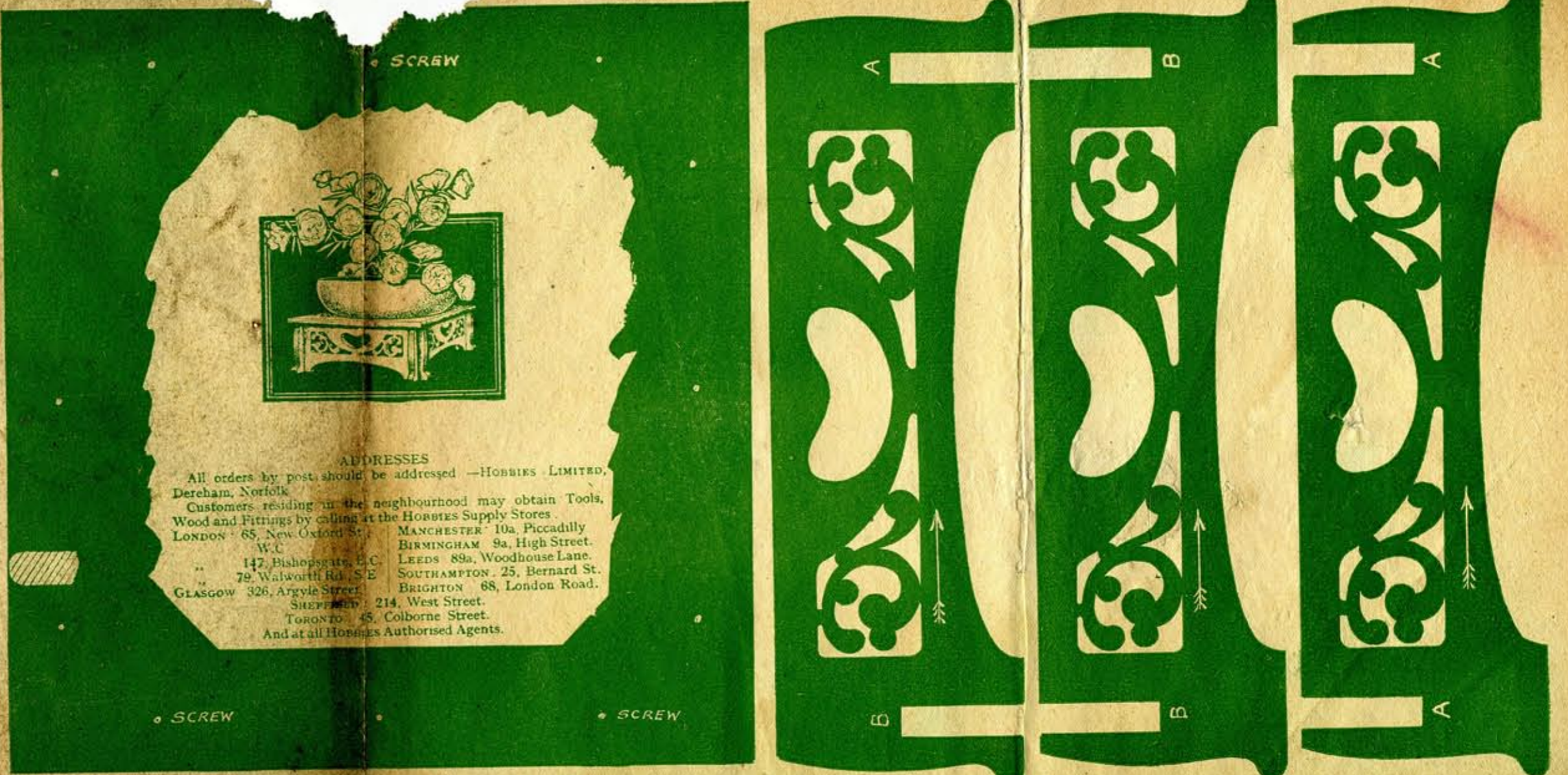
BOWL STAND, TOP.—Cut one 1/4 in. thick. Screw to the sides with round head brass screws. Round off the four edges as section if desired
