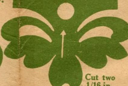
The → indicates direction of grain of wood.
