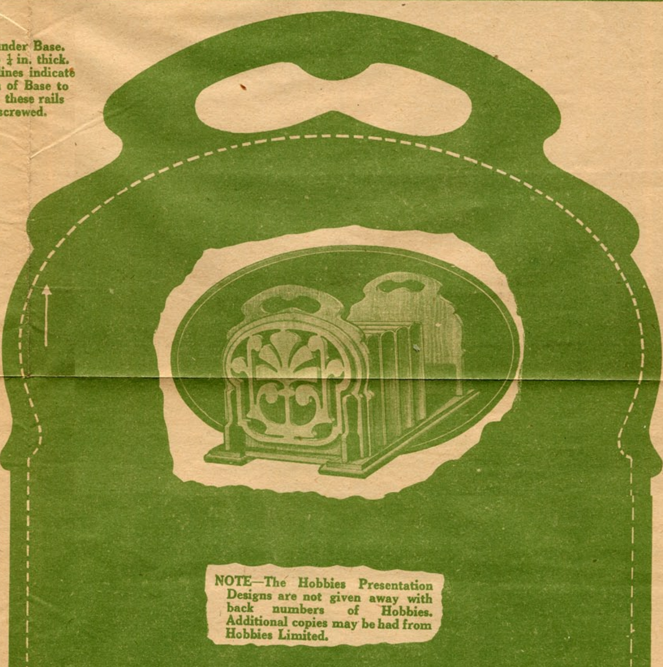
Solid End. Cut one ¼ in. thick and glue the Antofret panel on as shown by dotted lines.
