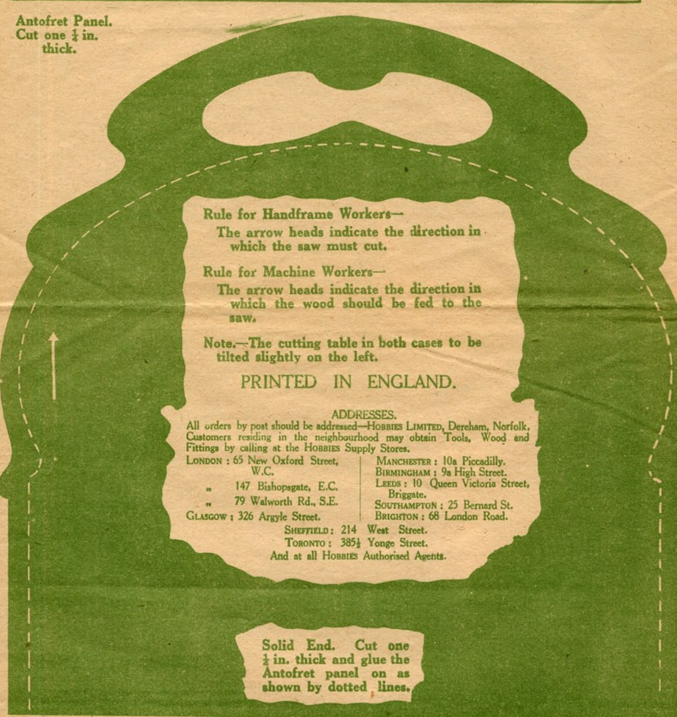
Solid End. Cut one ¼ in. thick and glue the Antofret panel on as shown by dotted lines.
