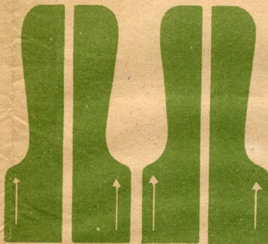
Uprights B glued to Antofret Panels. Cut from ¼ in. wood.
