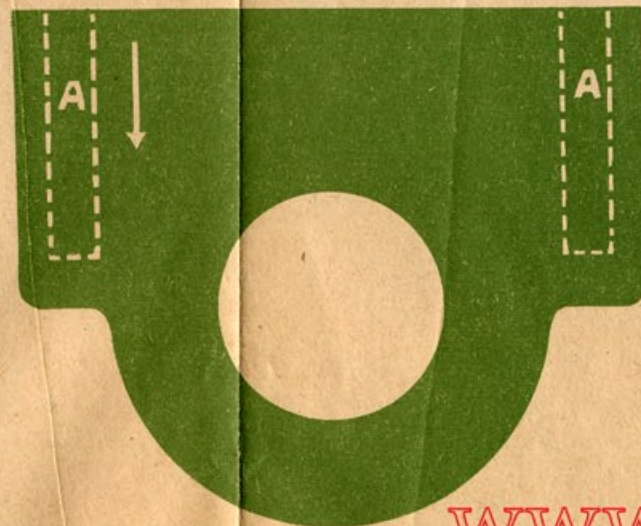
Vase Support. Cut one 1/4 in. thick.
