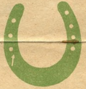
Horseshoe Overlays through which pass the ribbons connecting the Calendar Pad. Cut one of each 3/16 in. thick.
