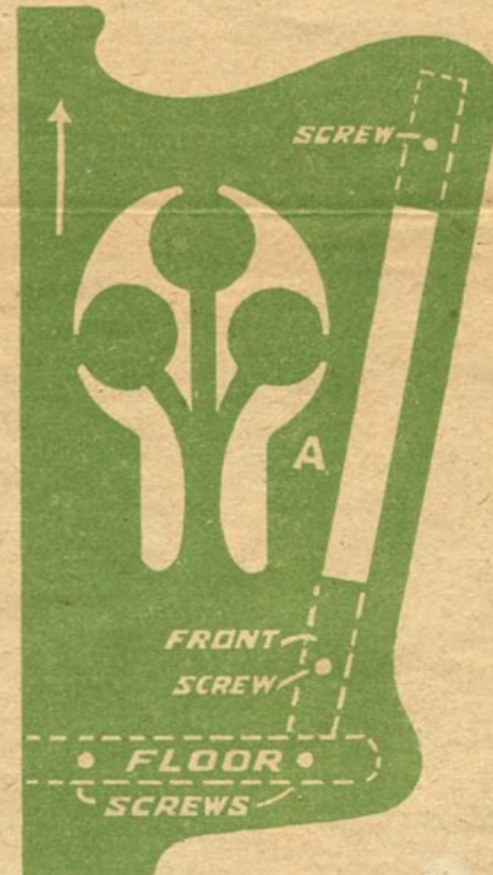
Side Bracket. Cut one 3/16 in. thick.
