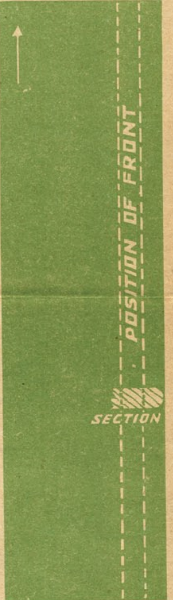
Floor of Letter Pocket. Cut one 3/16 in. thick. Round off front edge as shown by section.
