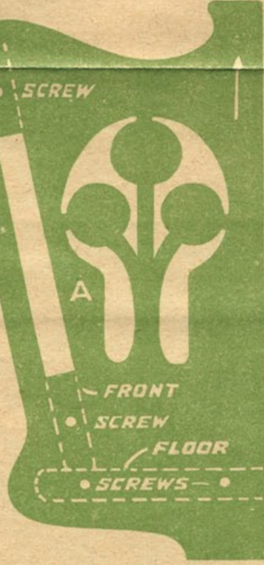
Side Bracket. Cut one 3/16 in. thick.
