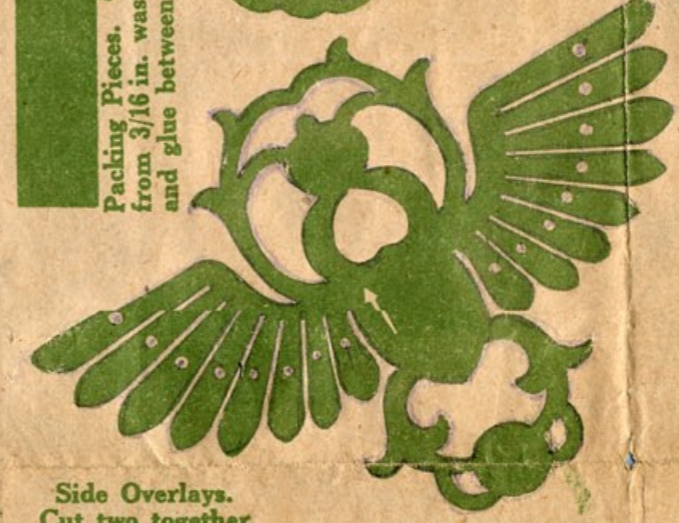
Side Overlays. Cut two together 1/2 in. thick.
