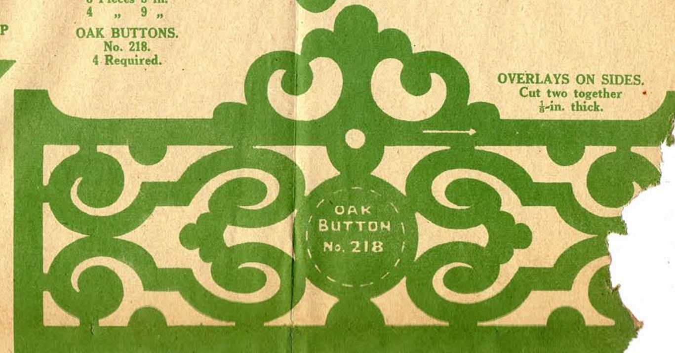
OVERLAYS ON SIDES. Cut two together \frac{1}{2} -in. thick.
