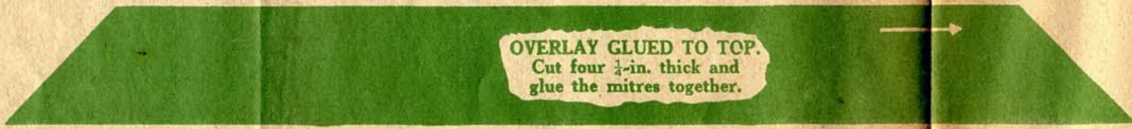
TOP OF JARDINIERE. Cut four \frac{1}{2} -in. thick and glue mitres together. Shape front edge to section shown.
