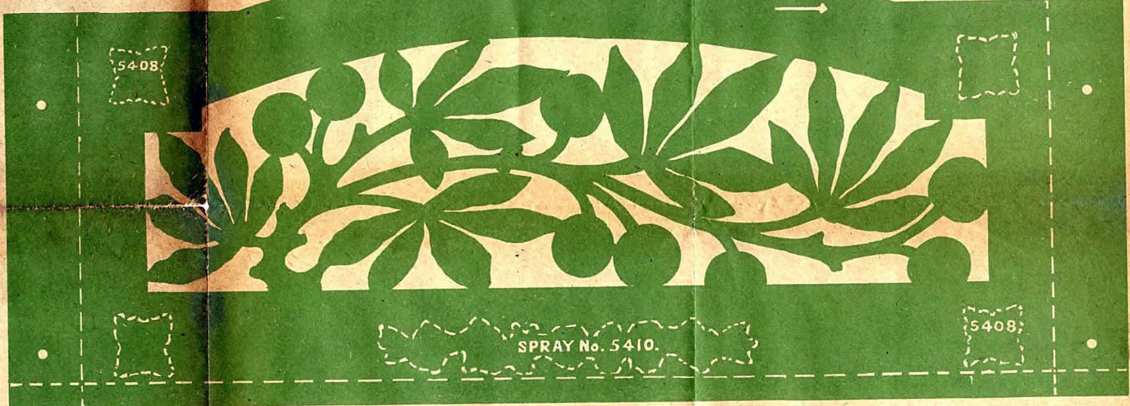
SIDE. Cut one 1/2 in. thick. Screw the sides and ends to the floor.
