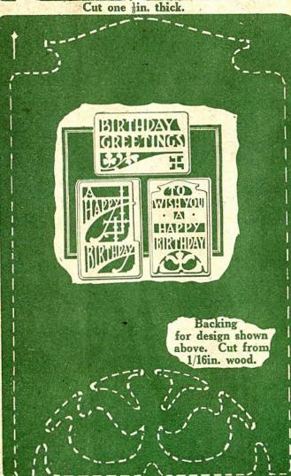
The backs of the fretted cards should receive the glue when putting on the thin backing wood. They should be put under weights until glue has
